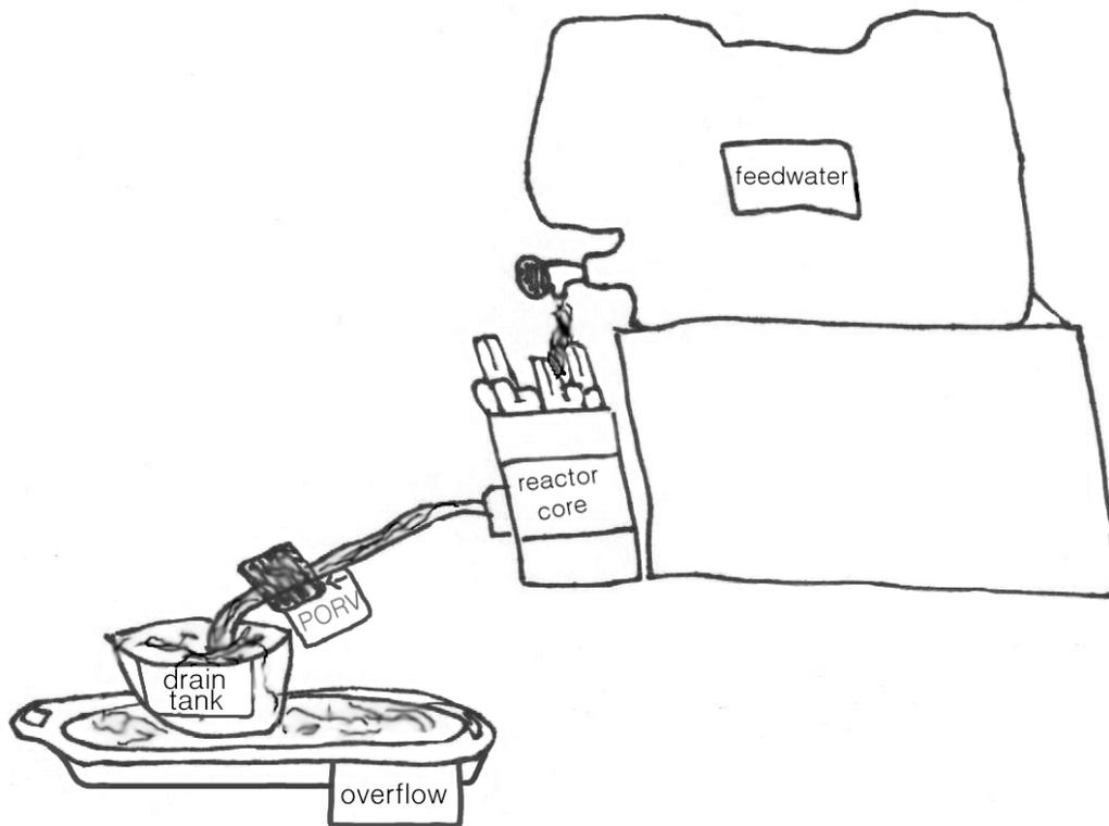
Set up model of nuclear reactor: Poke hole on side of cut milk carton, approximately 5 cm. from bottom. Push plastic tubing slightly into the hole and secure with duct tape. Place other end of tubing into empty bowl. Set thermos with water, or water container with valve, above the milk carton. Fill milk carton with 2 different colored straws to simulate fuel rods and control rods.
