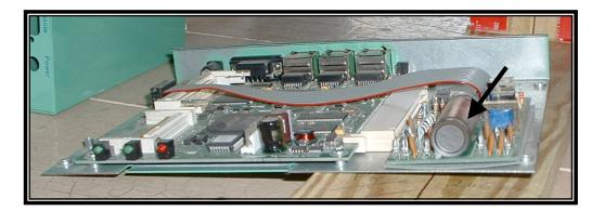
The LND 71210 GM radiation detector responds to x or gamma radiation, but does not respond to alpha or beta radiation. A typical gamma response for this detector is about 1,080 counts per minute per mR/h (Co-60). The full list of specifications for the LND 71210 detector is shown below (from LND web site).
