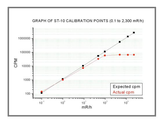
Calibration results for a group of ST-10 radiation monitors are shown in the following graph. Here, fifteen different units are calibrated and the results are then graphed. While differences are expected between individual units, in general there is only about a 10% difference in count rate between the lowest responding and highest responding ST-10 monitors (see following graph). It is expected that additional units other than the ones shown below, will provide similar results.
