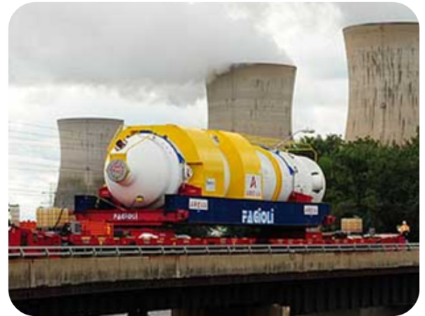
One of two new steam generators crossing the bridge to Three Mile Island .
