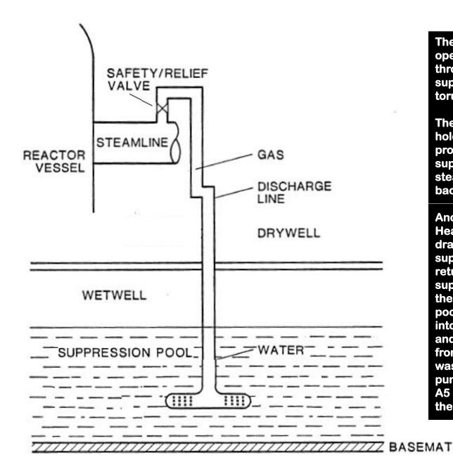
The steam flowing through an open safety relief valve travels through a pipe into the suppression pool (also called torus and wetwell).
