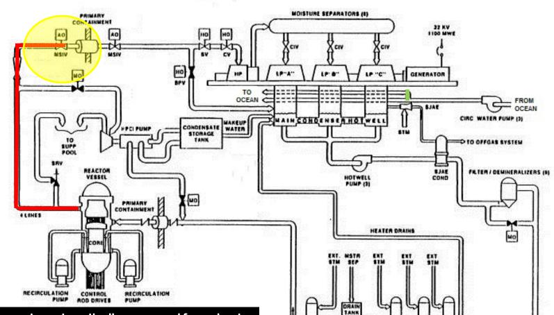
The reactor automatically scrammed from about 52% power when the second transmission line was lost. The de-energization of the switchyard and the trip of the main generator stopped the electric motors for the condensate, condensate booster, and circulating water pumps. The power loss also caused the main steam isolation valves to close, blocking the steam flow path to the main condenser.
