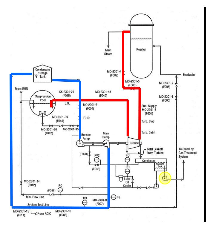
To control pressure inside the reactor, the operators ran the High Pressure Coolant Injection (HPCI) system. It takes steam from the reactor vessel to spin a turbine. The steam exits the HCPI turbines and flows into the torus.
