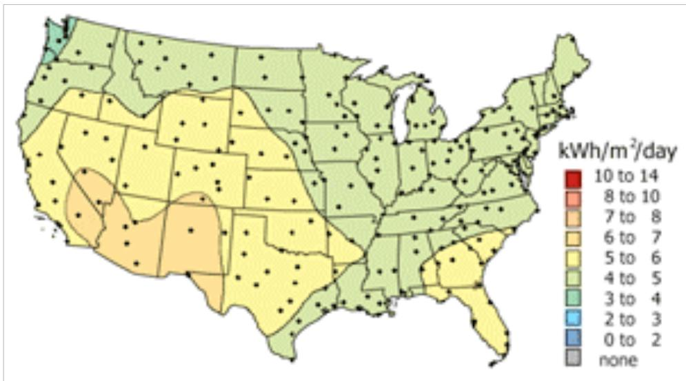
Annual average daily solar radiation per month, using a flat-plate collector facing south at a fixed tilt equal to the latitude of the site. Capturing the maximum amount of solar radiation throughout the year can be achieved using a tilt angle approximately equal to the site's latitude.
